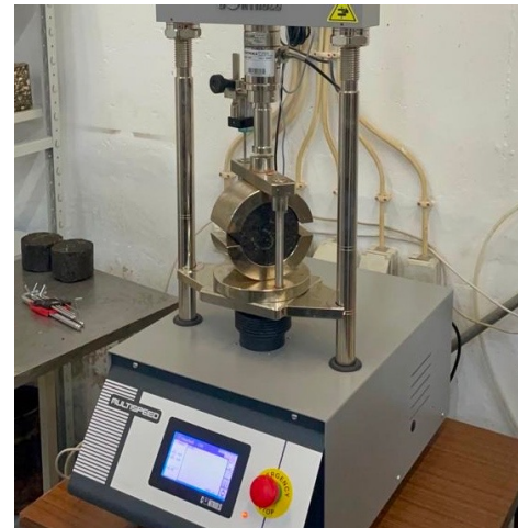
Marshall test @60°C
